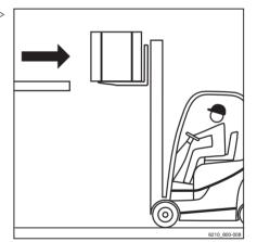
Lower the load while maintaining ground clearance.
