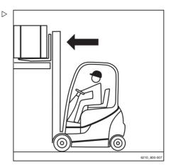
Lift the fork carriage until the load is resting pentirely on the fork.
