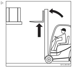
Insert the fork as far under the load as possible. Stop the truck as soon as the fork back is resting on the load. The load centre of gravity must be midway between the fork arms.
