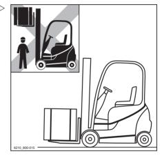
Lower the load until it rests securely on the rack.
